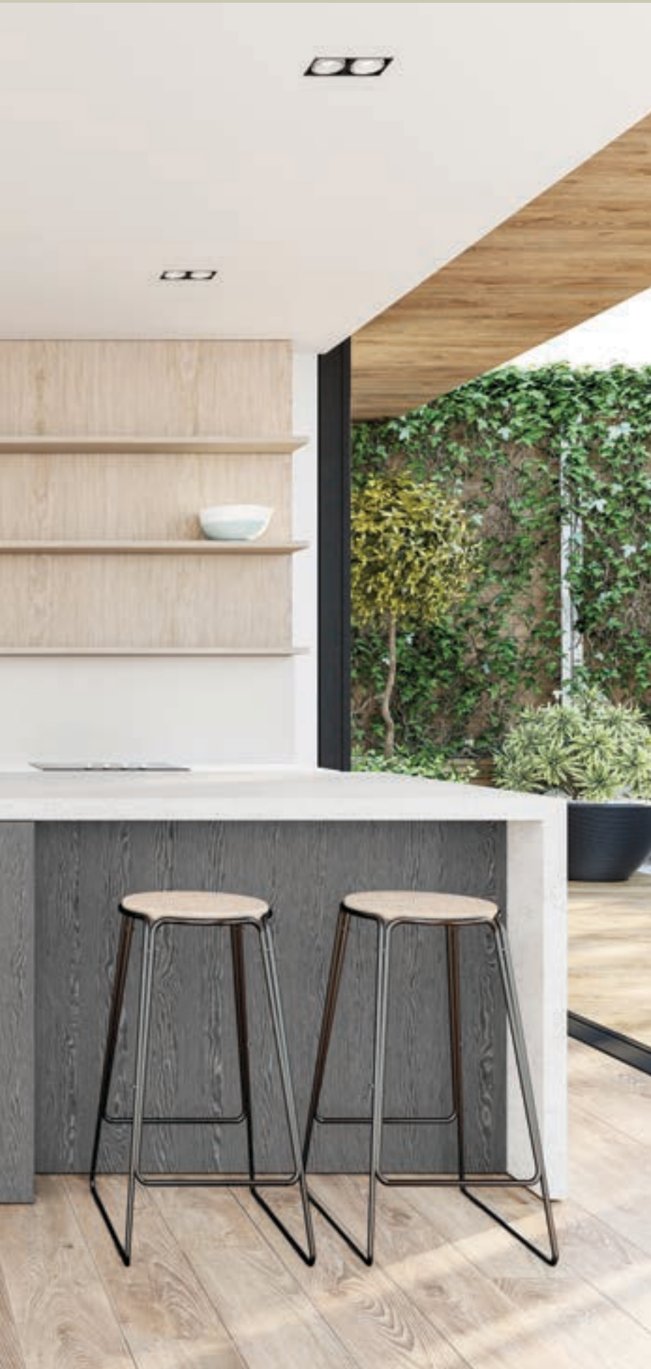
Island Cabinetry – Laminex Timber Veneer Reconstituted Smoked Greige, Planked, Clear Satin Finish; Back Wall and shelving – Laminex Timber Veneer Reconstituted Chalked Ash, Crown Cut, Clear Satin Finish; Benchtop – Caesarstone, Bianco Drift; Splashback – Laminam Bianco Assoluto.
